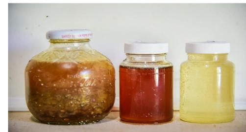
Figure 9: Oil samples taken from three different stages of AD. (Left) the influent, (middle) the effluent from primary digestion, and (right) the effluent from secondary digestion.
