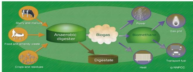
Figure 2: A schematic overview of anaerobic digestion
