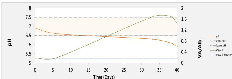
Figure 8: A comparison of alkalinity and pH collected from the CSD anaerobic digester over the span of 40 days. The ideal pH ranges are indicated on the graph (6.5 – 7.5).
