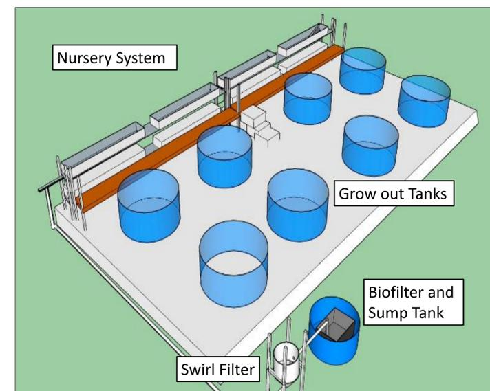
Figure 2. Sketchup showing all elements of the design
