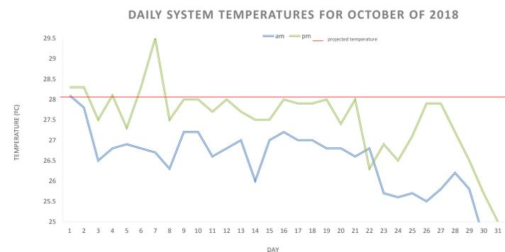
Figure 3. Temperature fluctuations for the month of October experienced in the Island School system. (Actual AM/PM Temperatures : Blue and Green Lines, Predicted AM/PM Temperature with heater: Red Line)
