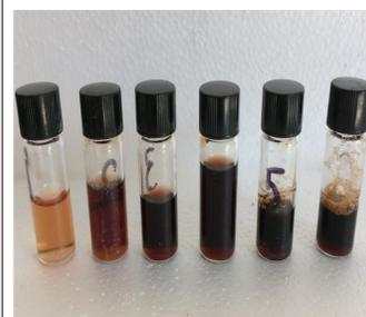
Image 9: Black liquor samples collected during the soda cook. The transition from white to black liquor over reaction time is evident with change in liquor color; indicative of lignin dissolution and increasing liquor density.
