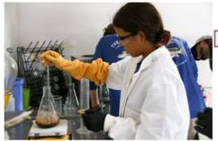
Image 2: Measurements being taken for density and pH of black liquor during the soda cook
