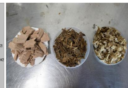
Image 10: Depiction of the Casuarina in the different stages of the soda pulping cook. The left sample is the Casuarina woodchips, the middle sample is partially digested woodchips, and the right sample is washed Casuarina soda pulp.
