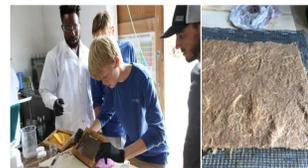
Image 4: Pressing pulp sheet to remove water to create a thinner sheet
