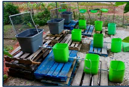
Image 1: Current prototype of the treatment systems built and constructed with 85% recycled material found at the Island School.
