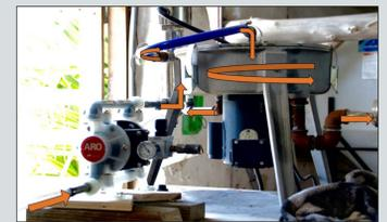
Image 4: Diagram of how WMO flows through the centrifuge.
