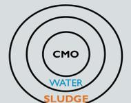
Figure 2: Top view of centrifuge
