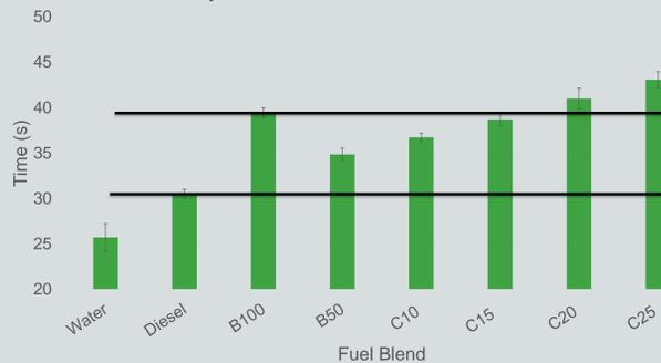
Figure 5: Fuel blend relative viscosities based on flow rate.
