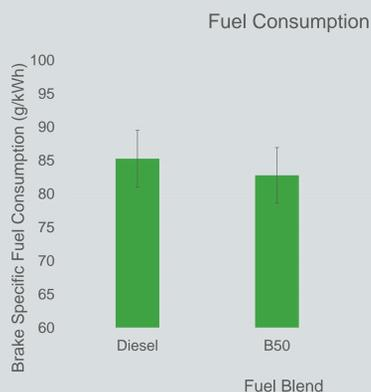
Figure 4: Brake Specific Fuel Consumption for select fuel blends.
