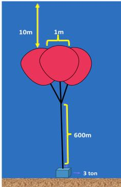
Fig. 3. The structure of a FAD deployed by the Cape Eleuthera Institute in the Northern Exuma Sound
